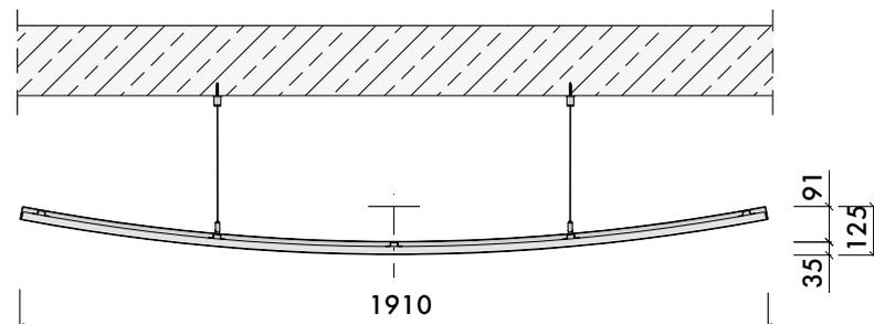
Ceiling rafts are delivered in one piece making them quick and easy to install. Flexible design and adjustable to various heights using steel cables.
