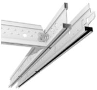
**Silhouette XL<sup>2</sup>** is designed to create a crisp, clean look to provide an enhanced aesthetic. The channel profile finishes flush with the ceiling surface leaving a minimalist 3mm or 6mm reveal.
